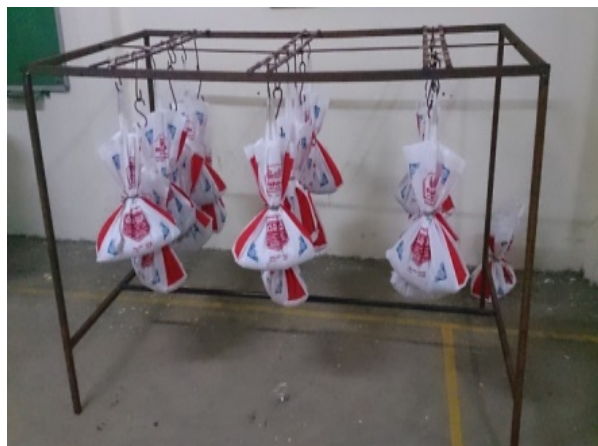
Fig. 2: A view of composites subjected to different loads
